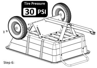
Position the tires onto the axle and place a machinery bushing over the axle and against the tire hub. Use a cotter pin to hold the wheels in position.
