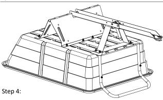
Position the tongue assembly on the axle housing and the yoke brace so that the tongue latch is facing forward and pointing downward.
