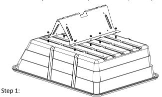
Turn the hopper upside down for ease of assembly. Bolt axle housing to the underside of the hopper, using the 3/8" round head screws.
