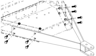
Bolt the tongue to the pump end of the skid using (8)  $3/8" \times 1"$  hex lock screws and hex whiz lock nuts (4 per side).
