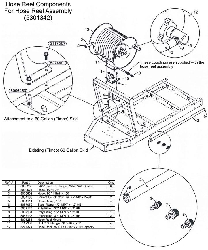
These fittings and hose/hose clamps may or may not be used, depending on what setup you are connecting this hose reel assembly to. Consider these as extra parts, if needed.
