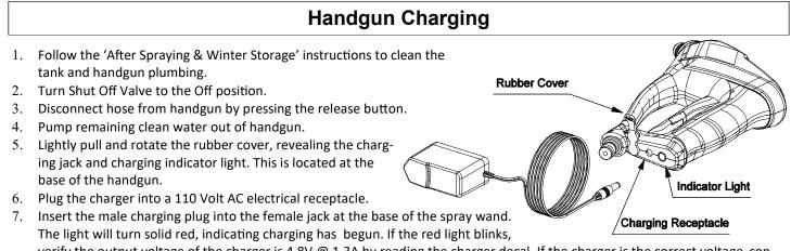
verify the output voltage of the charger is 4.8V @ 1.3A by reading the charger decal. If the charger is the correct voltage, continue charging and it will become solid red within 10 minutes. If the light continues to blink, the charger is the incorrect voltage and should be disconnected.
