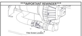
This sprayer comes with an On/Off valve located on your intake line. You must make sure the valve is in the "open" position before using your sprayer.
