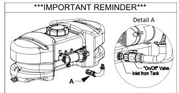
This sprayer comes with an On/Off (shut-off) valve located at the inlet location of the tank, towards the underside. (See Detail A). Make sure the valve is in the "open" position before using this sprayer.
