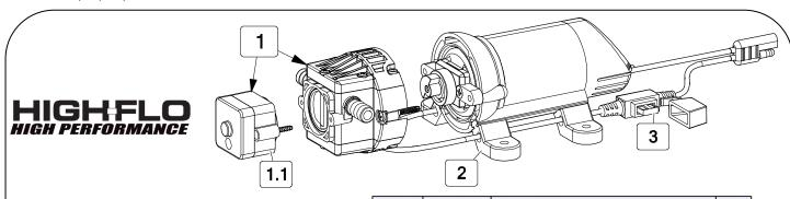
Pump Model: 5281370 1.2 GPM - 60 PSI Available Replacement Parts Replacement Pump: 5151086
