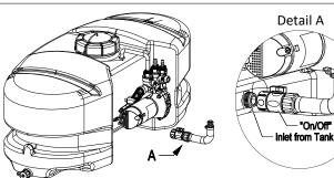
This sprayer comes with an On/Off (shut-off) valve located at the inlet location of the tank, towards the underside. (See Detail A). Make sure the valve is in the "open" position before using the sprayer.
