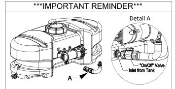
This sprayer comes with an On/Off (shut-off) valve located at the inlet location of the tank, towards the underside. (See Detail A). Make sure the valve is in the "open" position before using sprayer.
