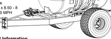
Caution: When fully filled with water, this sprayer will weigh approx. 745 lbs.. Consult the owner's manual for your vehicle to verify that you are within it's load carrying capacity.
