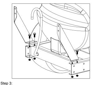
The left & right boom mounting brackets are to be mounted on the trailer frame. Use 4 bolts and nuts to secure them in place.
