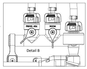
method to set the pressure is to open the boom valve completely and if a lower pressure is desired, then slowly open the bypass valve until that pressure is obtained.
