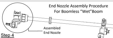
Boom will come with the (2) end nozzle assemblies NOT affixed to the boom tube. Follow the instructions below to attach these properly to the boom tube, as shown.
