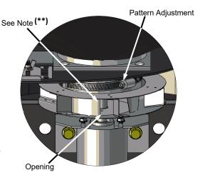
NOTE: To return the pattern adjust ring to the factory setting, simply align the pattern adjust ring to the center of the mounting plate, as pictured above (\*\*).
