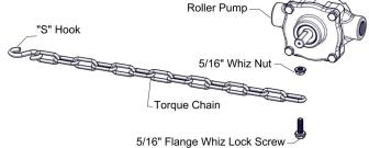
\*\*\* Insure that this connection point will not allow the roller pump to spin on the PTO shaft \*\*\*
