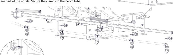
Loosely slide a hose clamp on to the feeder hose, connect the boom feeder hose to the hose barb tee on the nozzle harness and secure with the hose clamp.
