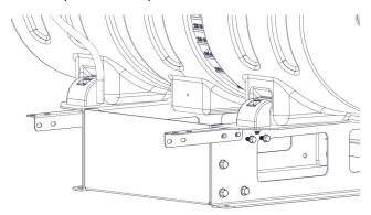
Now, attach the nozzle harness to the boom with the nozzle clamps and the nozzles to the inside of the fold, pointing down.
