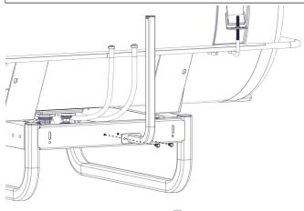
1. Attach the Upright Boom Mount to the 3PT tube frame, using (2) hex bolts and (2) nuts.
