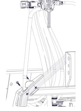
Attach the Manifold Bracket to the 3PT Frame using (2) bolts and nuts.
