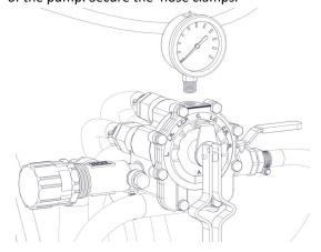
7. Using a sealant or plumber's Teflon tape, thread the gauge into the top of the tee valve assembly.
