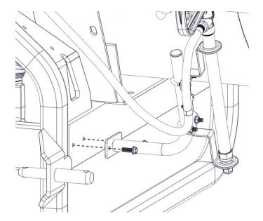
Install the hose wrap mount (handgun/hose bracket will already be attached to the mount) to the sprayer frame using (2) bolts and nuts.
