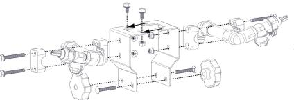
2. Assemble the Broadcast Nozzle Mounts and Nozzles, as shown, if not already done.
