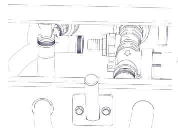
3. Connect the 3/4" x 42" bypass hose to the 3/4" hose barb on the strainer assembly and tighten hose using a 3/4" hose clamp from the parts bag. The hose will already be secured to the valve manifold by the factory.
