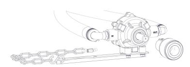
6. The roller pump <u>IS</u> included with the assembly. Attach the adapter, the torque bracket, torque chain, S-hook, lock washers, hex bolts and the rapid/quick link to the pump as needed. It is intended for your pump to be mounted directly to the tractor PTO. The torque chain needs to be secured to the tractor to keep your pump from spinning.
