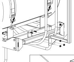
8. Attach the boom buster bracket to the telescoping brackets, using the two square u-bolts and 4 whiz nuts. The telescoping brackets are already mounted to the 3-point frame.
