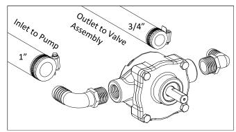
4. Using a good quality thread sealant, thread the 1" fitting into the inlet (IN) side of the pump and the 3/4" fitting to the outlet (OUT) side of the pump. With a twisting motion, attach the other end of the 1" hose to the 1" fitting on the inlet to the pump. Slip a 3/4" hose clamp onto the 3/4" hose coming off the valve assembly and with a twisting motion, attach the 3/4" hose to the output side of the pump and securing with the hose clamp.
