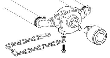
5. The roller pump IS included with the assembly. Attach the adapter, the torque chain and S-hook to the pump as needed. It is intended for your pump to be mounted directly to the tractor PTO. The torque chain needs to be secured to the tractor to keep your pump from spinning.
