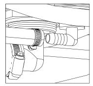
Slide a hose clamp on to the bypass hose (from the relief valve), then with a twisting motion, slip the bypass hose over the fitting on the bottom of the tank. Slide the hose clamp to the end of the hose and secure.
