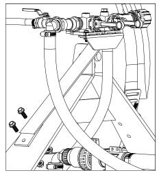
1. Install the preassembled tee valve sub-assembly to the 3-point carrier valve mount and position as shown.
